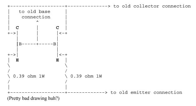
The 0.39-ohm resistor allows the transistors to be hooked in parallel without one transistor going into thermal runaway and trying to drive the whole load itself. (A good place to find out more about hooking transistors in parallel is a Voltage Regulator handbook of some kind)
